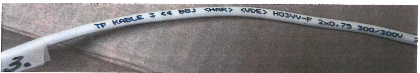
Picture 2. Cable 3 marking
